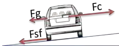
Figure 2 Forces related to the mechanism of skidding
