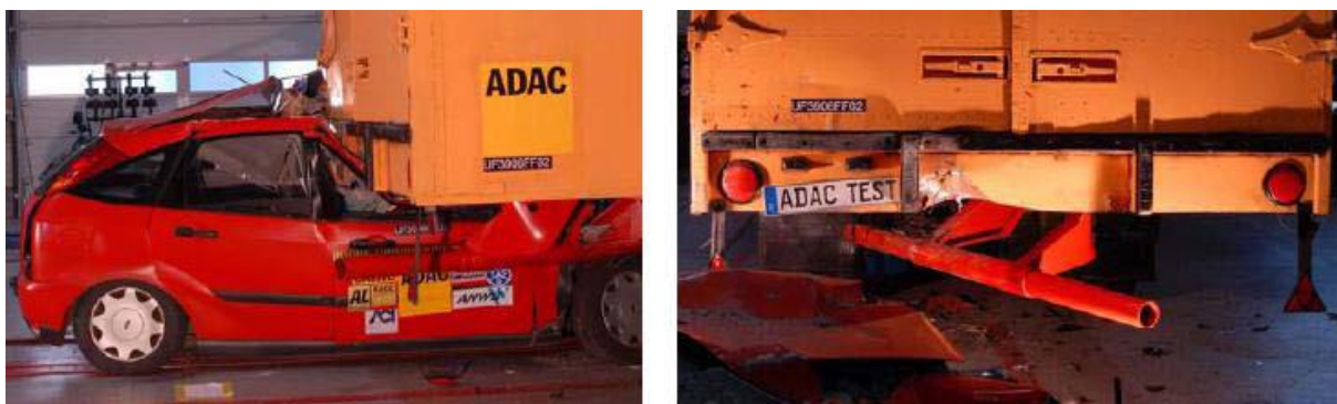
Figure 1: Results of ADAC crash test with underrun protection conforming to 2006/20/EC [from Smith et al. 2008, ADAC 2006]
