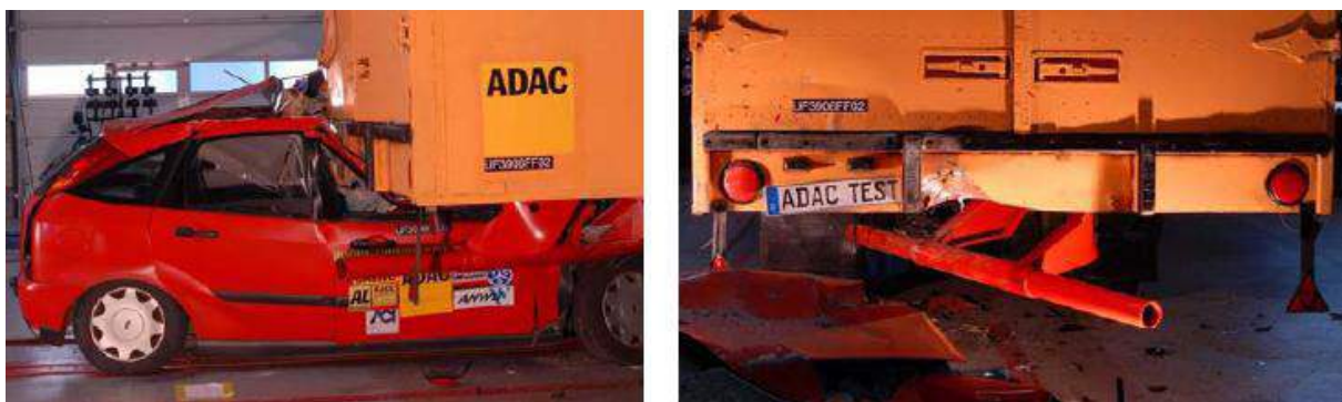
Figure 7: Results of ADAC crash test with underrun protection conforming to 2006/20/EC [from Smith et al. 2008, ADAC 2006]
